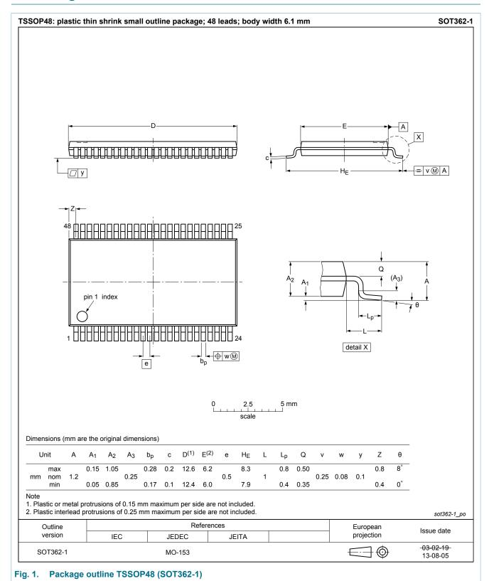
plastic, thin shrink small outline package; 48 leads; 0.5 mm pitch; 12.8 mm x 6.1 mm x 1.2 mm body
